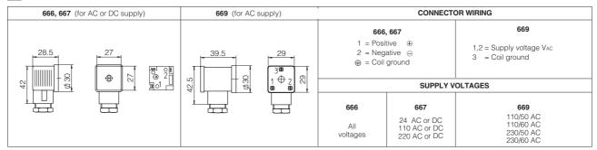
Note: for electronic connectors type E-SD, see tab. K500
